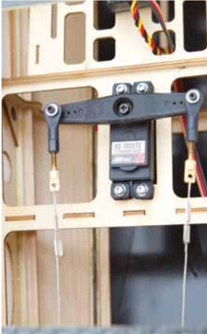
Ball linkages and double control horns ensure tight and efficient control system responsiveness.
