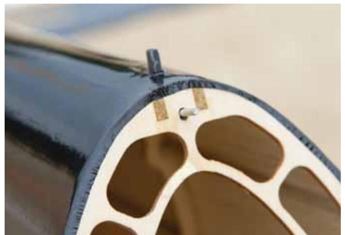
**A spring-loaded mechanism in addition to magnets keeps the canopy in place during high-energy aerobatics. This airframe has lots of lightening holes.**
