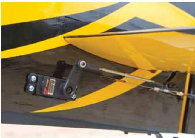
**A powerful Hitec servo, a large servo arm and the pull-/pull rudder offer incredible yaw authority.**
